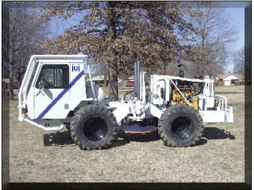
Side View Dimensional Drawing of the 'minivib' II mounted on the 'minibuggy'
